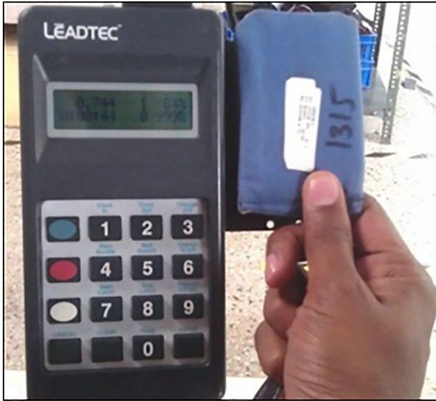
Figure 1. Technology-Enabled Quantification of Work: RFID Scanners Installed on Treated Lines
